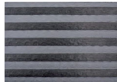
Section of a recycled panel with tape reinforcement.
