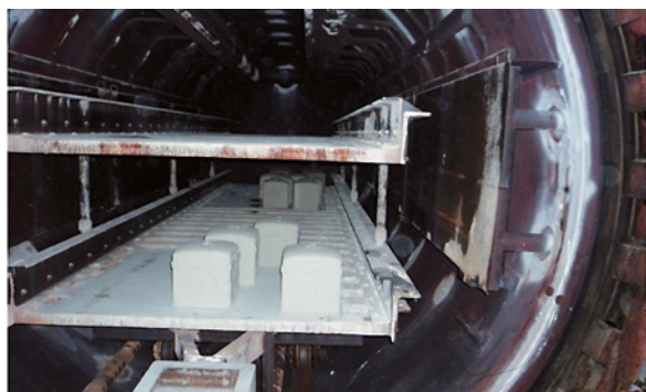
AAC small-scale test specimen after hydrothermal curing
