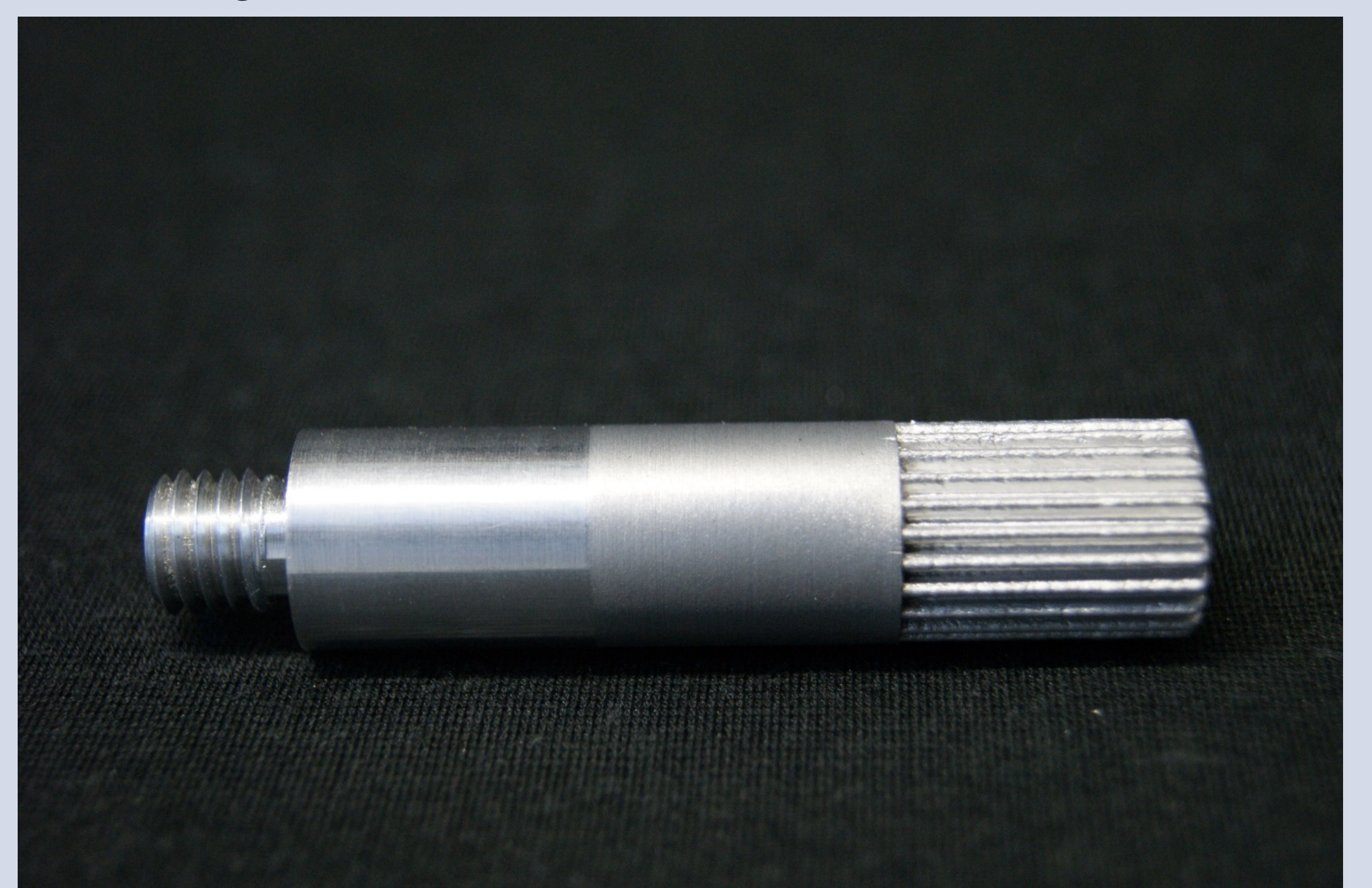
Reparatur mittels Additive Repair (© IPeG, Uni Hannover)
