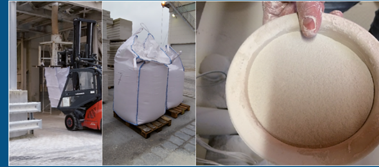
Powder from post-demolition AAC.
