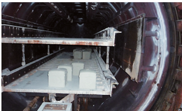
AAC small-scale test specimen after hydrothermal curing
