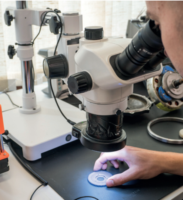
Fig. 7: Additively manufactured gear wheel of an electric bicycle motor (© Fraunhofer IPA)
